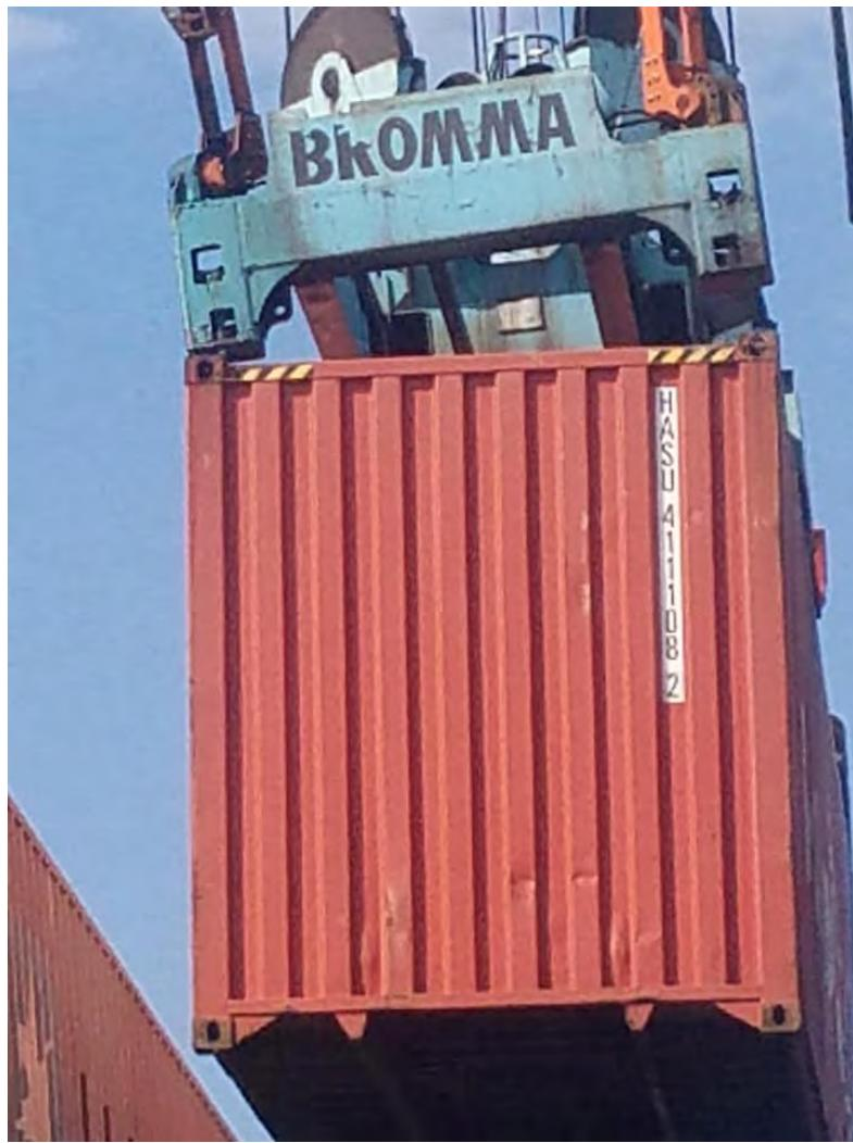
When engaging containers with any spreader device, check your equipment's console lights and get an indication about twist lock engagement. Then, just to be sure, take a test lift and float the load. When lifting containers, being locked into three corners isn't enough. Containers are designed to be top lifted vertically; from all four corners.
