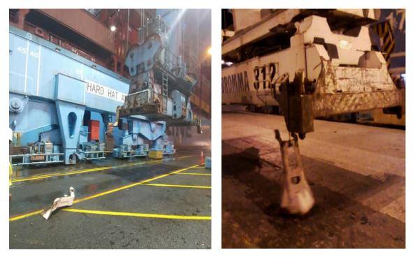
Conscientious condition and maintenance checks should typically provide enough insulation to effectively guard against the obviously dangerous container spreader flipper "free-fall", an example of which is shown in the photograph *above left*.
