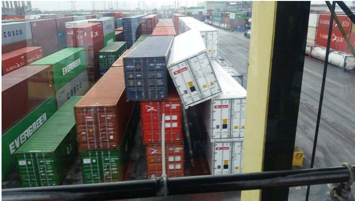
Lately, at ports up and down the East and Gulf Coasts, we've been observing a higher than normal number of poorly stacked, upper tier containers. That's obviously not good, in that containers that are not stacked corner-fitting-to-corner-fitting have a way of causing serious, life threatening hazards to the people we care the most about: **YOU!**
