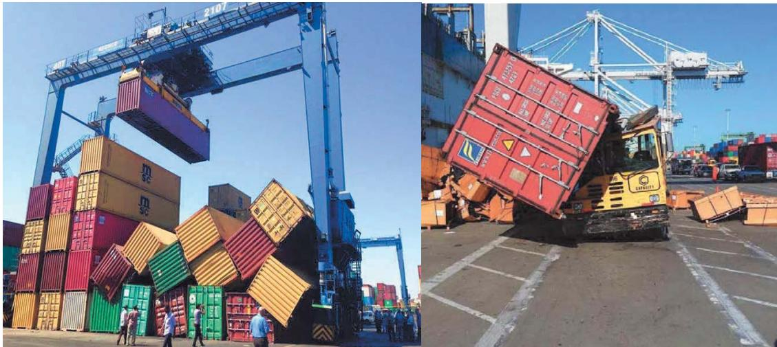
Globally, The ILA-USMX Joint Safety Committee has observed an increased incidence of stowed/stacked containers that are knocked out of position (toppled) by another container being trolleyed along the bridge of ship to shore or yard gantry cranes (RTGs).
